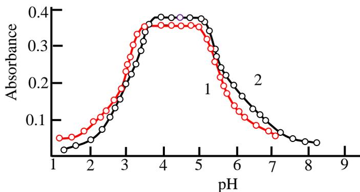
Fig. 1. Absorbance of Co- HNTPh -Am extracts function of the pH of the aqueous phase.
