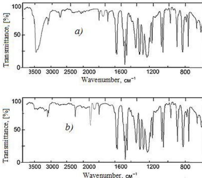
**Fig. 4.** IR spectrums of HNTPh (a) and the Co (II)- HNTPh-DPhA (b).
