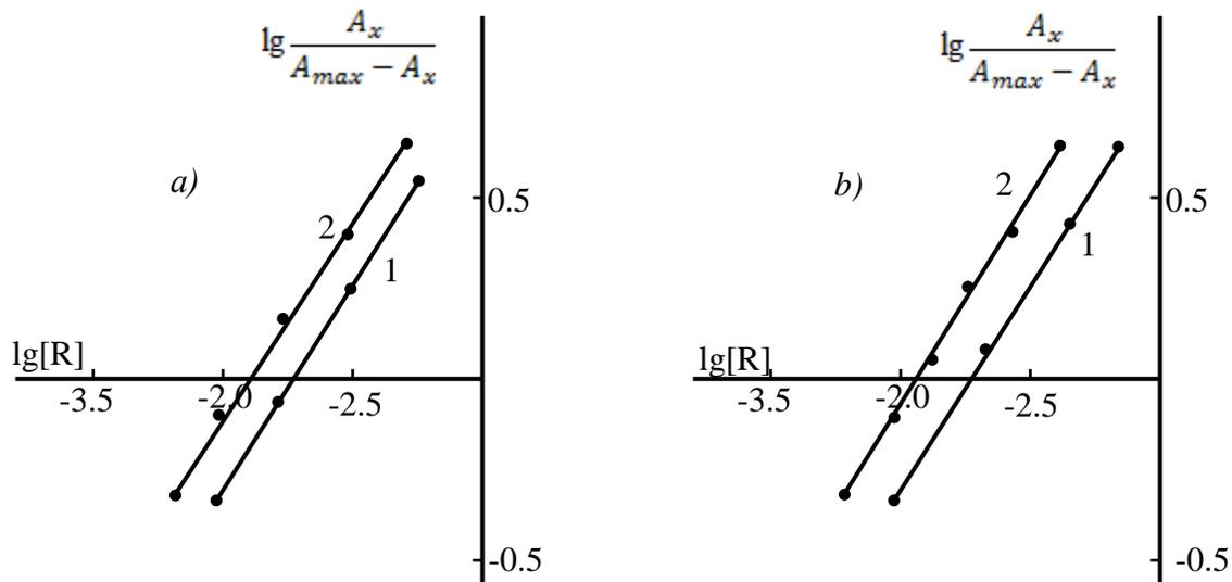
**Fig.3.** Determination of the ratio of components by the equilibrium shift method for (a) Co (II)-HNTPh-DPhA and (b) Co (II)- HNTPh-TPhA. 1- Co (II) : HNTPh; 2- Co (II): Am.
