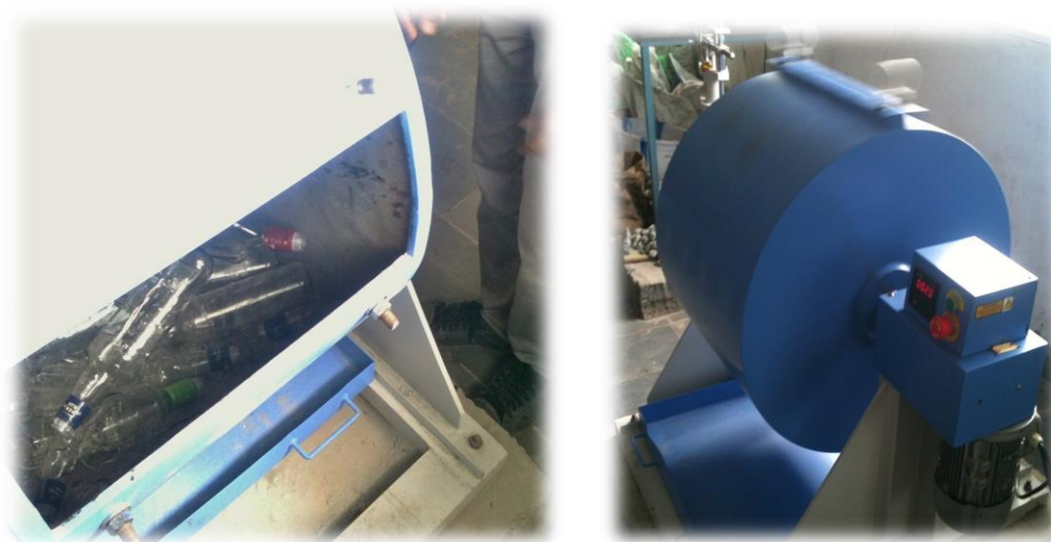
Fig 2:Crushing of waste glass in to powder by Los-Angeles abrasion machine
