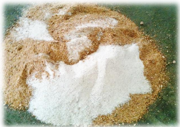
Fig 3: Partial replacement of fine aggregate with glass powder
